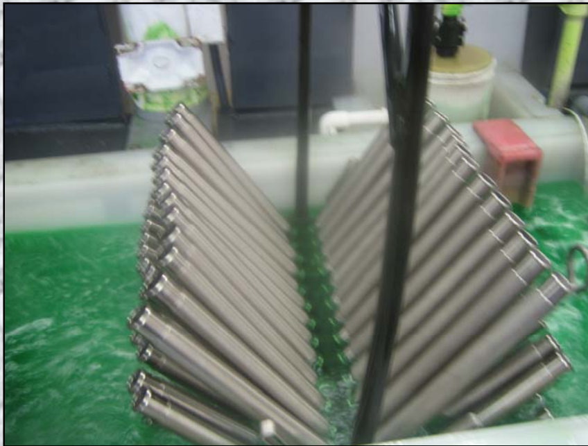
600 gallon Electroless Nickel line built by LeKem. Runs up to 10,000 parts a day.
