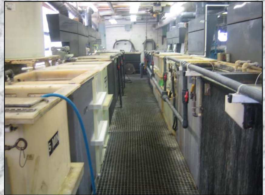
600 gallon Electroless Nickel line built by LeKem. Runs up to 10,000 parts a day.
