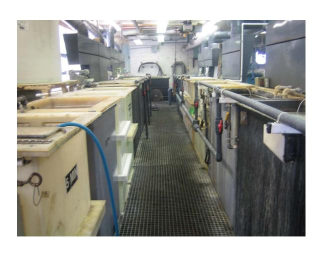
Print of plating shop that shows a horse shoe EN system (that is separate from all other plating) that plates up to 20,000 parts a day
